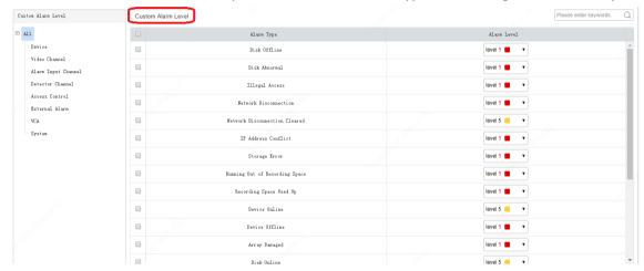
Or assign the same alarm level to multiple alarm types: select alarm types and then click **Custom Alarm Level**. In the dialog box displayed, select the desired alarm level and then click **OK**.
