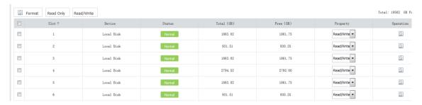
• When RAID mode is turned on with array(s) created, you can view array disk information, format disks, modify disk property. This page is empty when there is no array.
